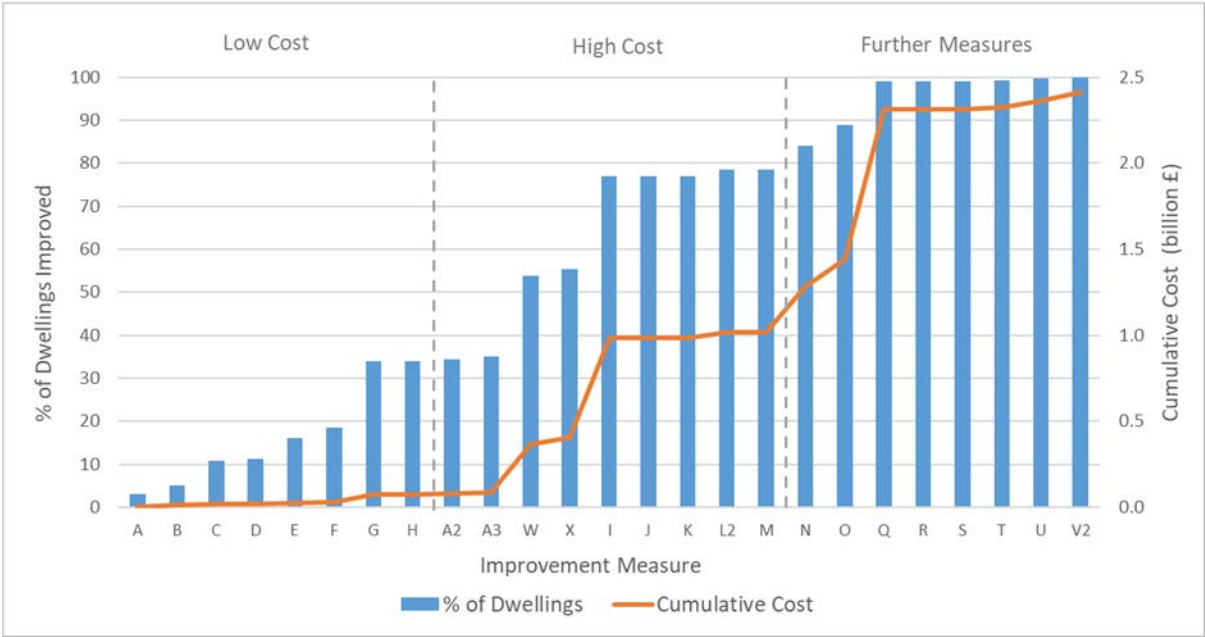
Figure 1: Percentage of dwellings improved to EER band C with each improvement, and the associated cumulative cost.
